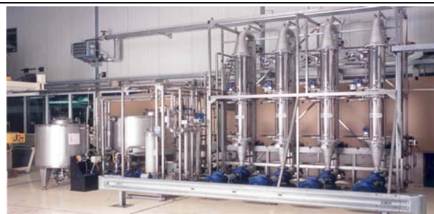
Figure 4. Microfiltration unit with a capacity of 20m 3 /h to separate softeners during the production of flat film (source: Amafilter GmbH).
