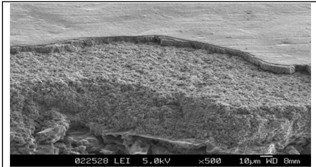
Figure 2. Scanning electron microscope image of the multi-layer membrane applied to the porous carrier material
