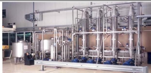
Figure 4. Microfiltration unit with a capacity of 20m<sup>3</sup>/h to separate softeners during the production of flat film (source: Amafilter GmbH).
